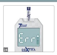
The following errors will be shown on the display with an 'Err' or 'EEE' notification:
