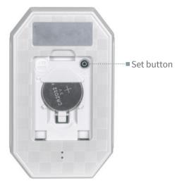
First remove the battery cover and check that the required 3 V lithium battery (type CR 2032) has been inserted. If this is not the case, you will need a new battery (see page 48).
